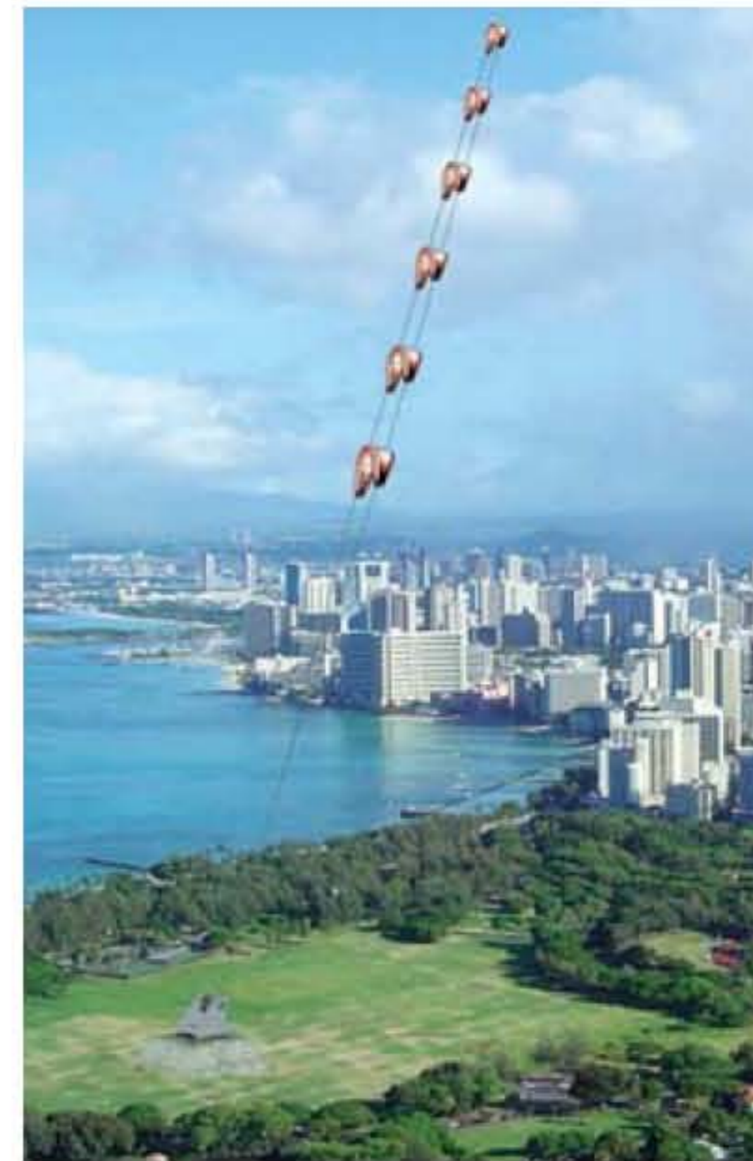
▲ Laddermill wind power system would string C-shaped kites (shown), parasails or flying wings along the upper half of a wire. Each wing would use sensors and actuators for steering and pitch control as it climbed and then descended. The scheme would allow heavy generators to remain on the ground.
