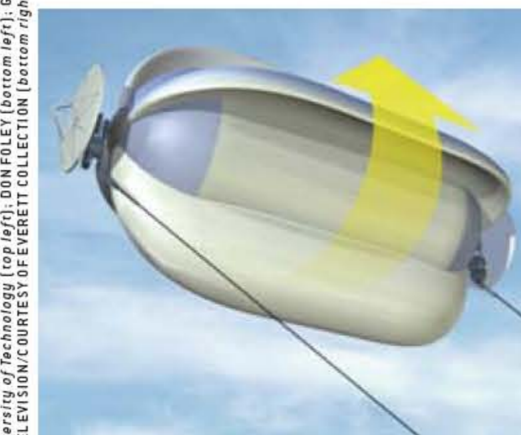
▲ Like a spinning blimp, a helium-filled rotor would catch the wind in fabric scoops, turning generators attached to tethers, which would then conduct the electricity to a transformer on the ground.
