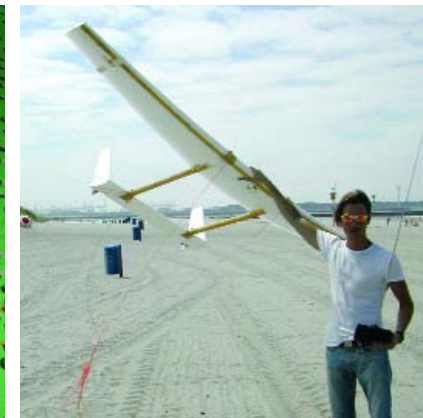
figure 4: The high L/D kiteplane. [source: J. Breukels]
