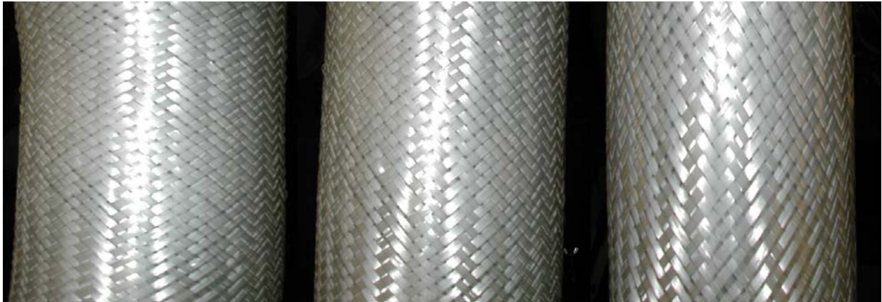
Figure 5. The re-orienting of free fibers under internal pressure (pressurized on the left, unpressurized on the right [Ref 1]
